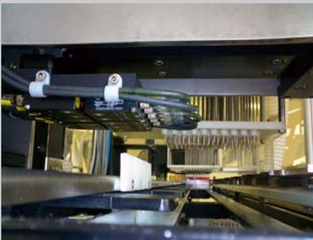
The Oysterbay saturation equipment siphons filled test tubes and refills them with an aqueous non-sterile solution. The equipment processes 60,000 tubes of different dimensions per hour. Trays of 50 are processed 2 at a time every 3 seconds.
